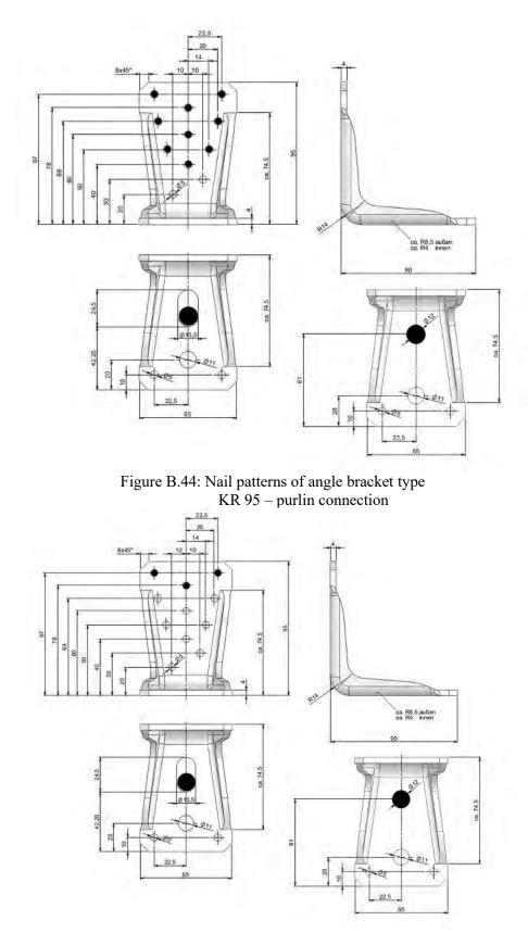
Figure B.45: Nail patterns of angle bracket type KR 95 – column connection
