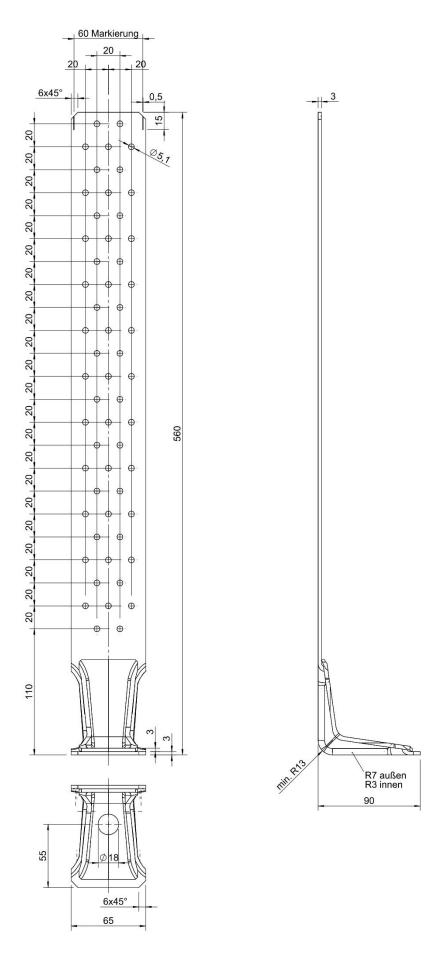
Figure B.2 Dimensions of type KR 560x90x65x3,0
