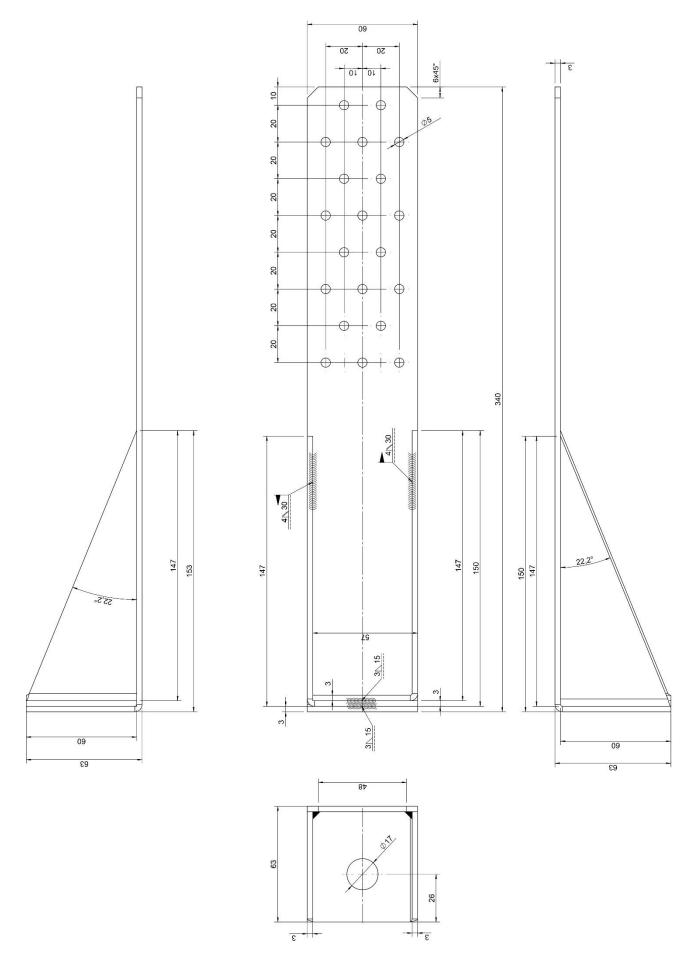
Figure B.5 Dimensions of type R 340x60x60x3,0 - alternative hole diameter 18 mm in bottom plate
