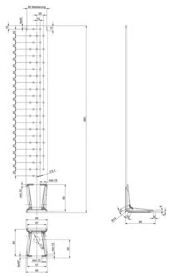
Figure B.4 Dimensions of type KR 560x90x65x4,0
