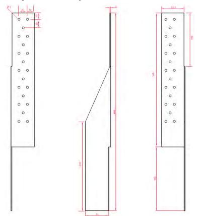
Figure B.19 Dimensions of vertical flange BPL465 S250 for two-piece hold-downs
