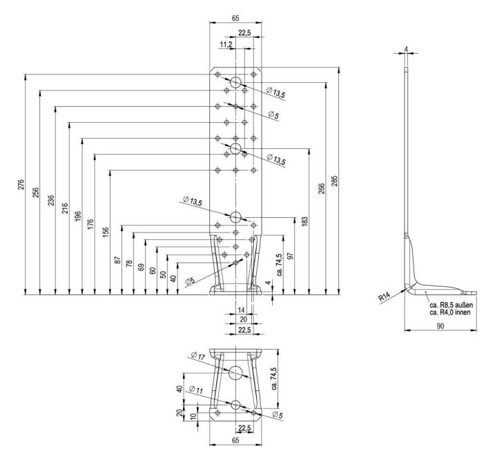
Figure B.43 Dimensions of type KR RL 285x65x4,0\_Ø17
