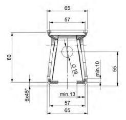
Figure B.3 Dimensions of type KR 460x90x65x4,0
