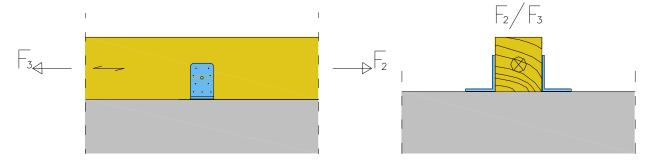
Figure B.25: Load F<sub>2</sub> / F<sub>3</sub>, purlin
