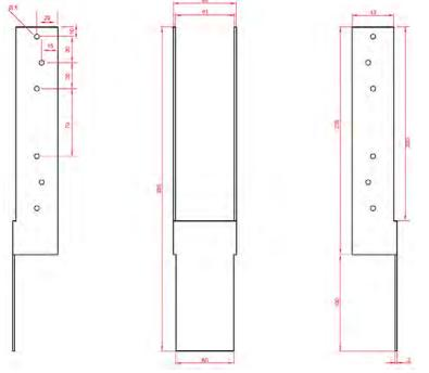
Figure B.16 Dimensions of vertical flange BPD S250 for two-piece hold-downs
