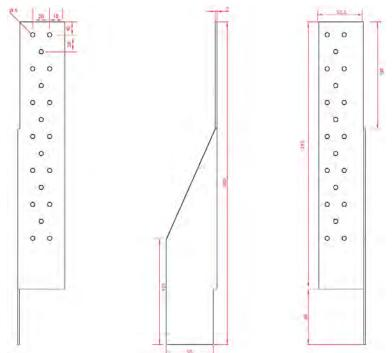
Figure B.17 Dimensions of vertical flange BPL380 S250 for two-piece hold-downs
