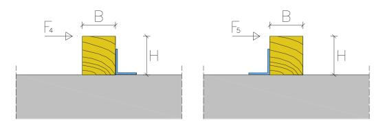
Figure B.26: Load F<sub>4</sub> (left) and Load F<sub>5</sub> (right)
