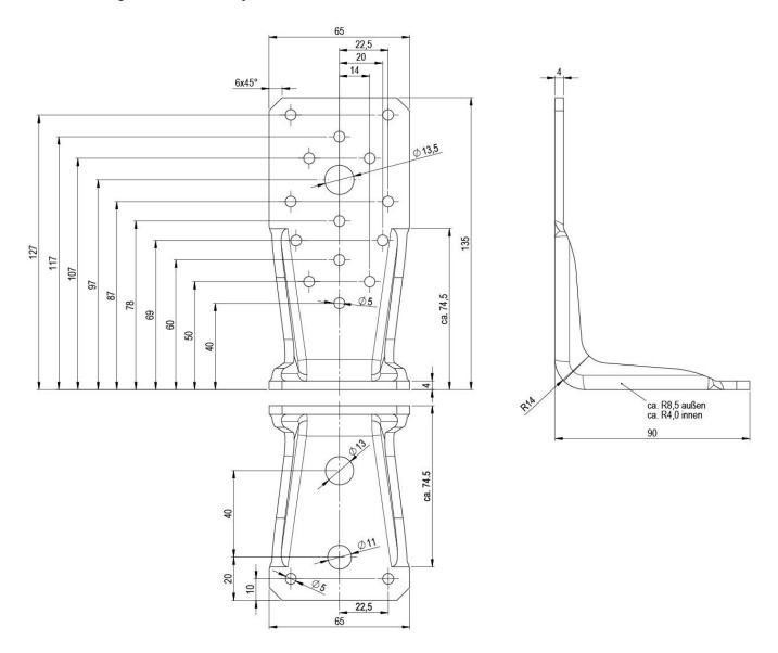
Figure B.38 Dimensions of type KR RL 135x65x4,0\_Ø13
