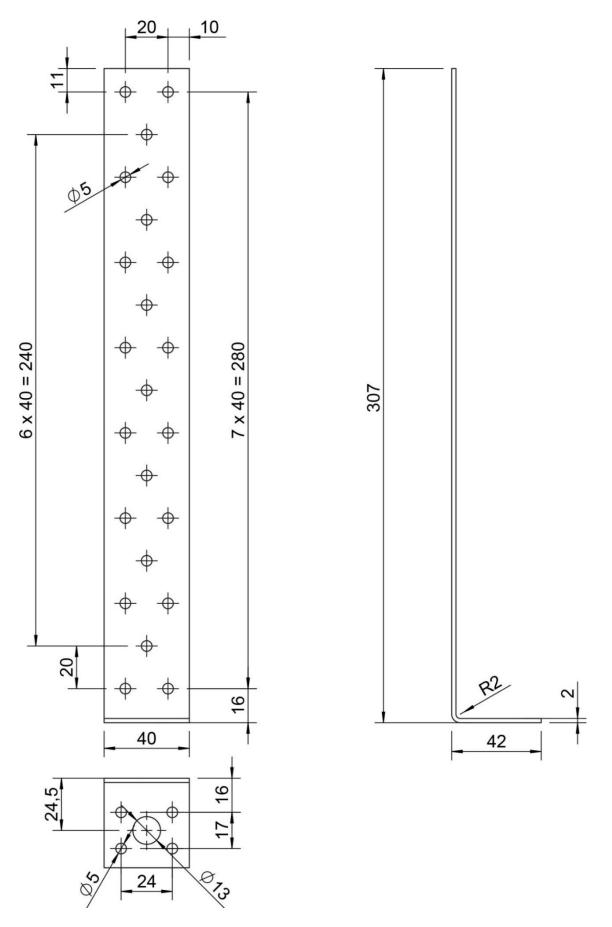
Figure B.53 Dimensions of concrete flat steel anchor 300x40x40x2,0
