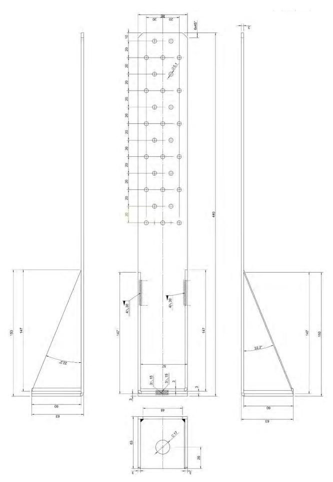
Figure B.6 Dimensions of type R 440x60x60x3,0 - alternative hole diameter 18 mm in bottom plate
