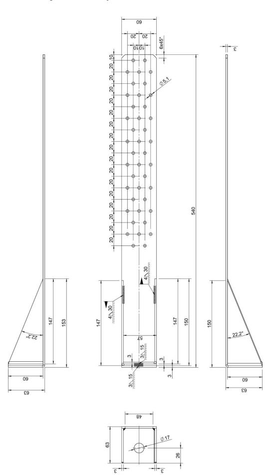
Figure B.7 Dimensions of type R 540x60x60x3,0 - alternative hole diameter 18 mm in bottom plate
