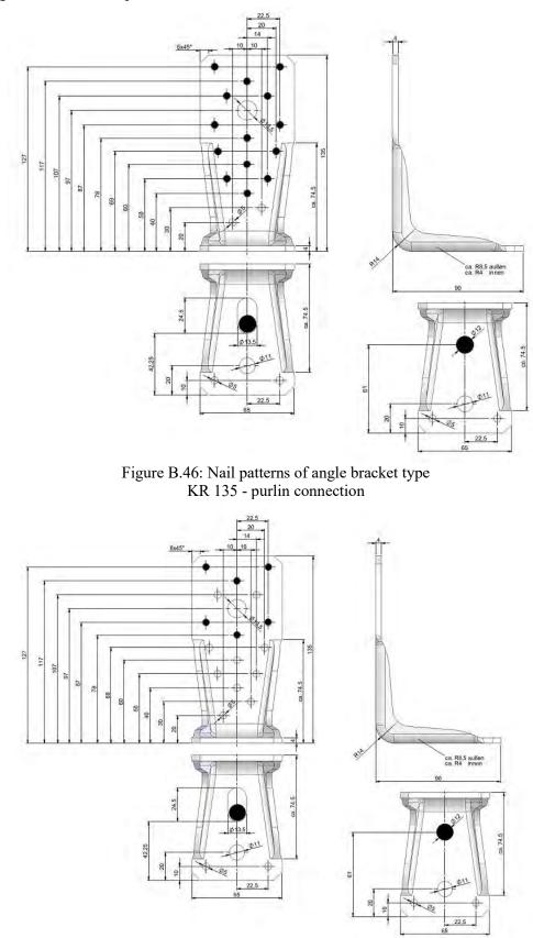
Figure B.47: Nail patterns of angle bracket type KR 135 - column connection
