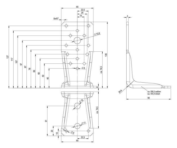
Figure B.37 Dimensions of type KR RL 135x65x4,0\_Ø12
