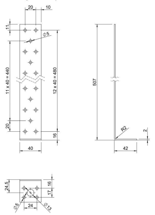
Figure B.57 Dimensions of concrete flat steel anchor 500x40x40x2,0
