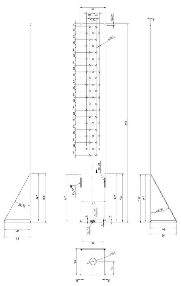
Figure B.8 Dimensions of type R 620x80x80x3,0
