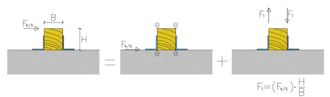
Figure B.27: Load Case  $F_4/\,F_5$  reduced to two basic load cases
