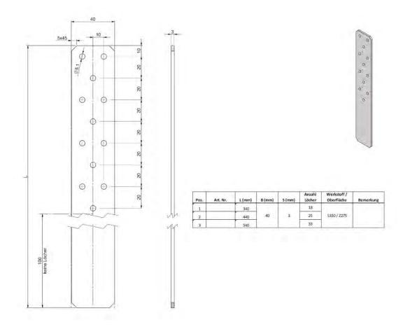
Figure B.15 Dimensions of 40 mm vertical flange for two-piece hold-downs
