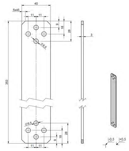
Figure B.22 Dimensions of storey connector 353x40x3 made of S355/Z275
