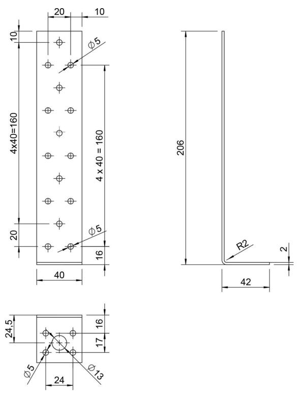
Figure B.51 Dimensions of concrete flat steel anchor 200x40x40x2,0
