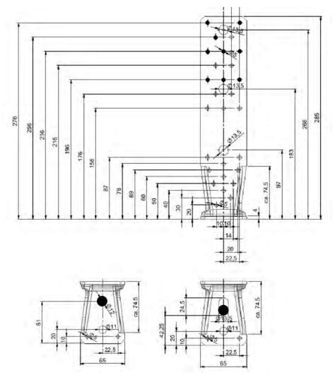
Figure B.50: Nail patterns of angle bracket type KR 285 - column connection
