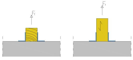
Figure B.24: Load F<sub>1</sub>, purlin (left) and column (right)
