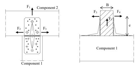
Figure B.23: Load directions and eccentricity e
