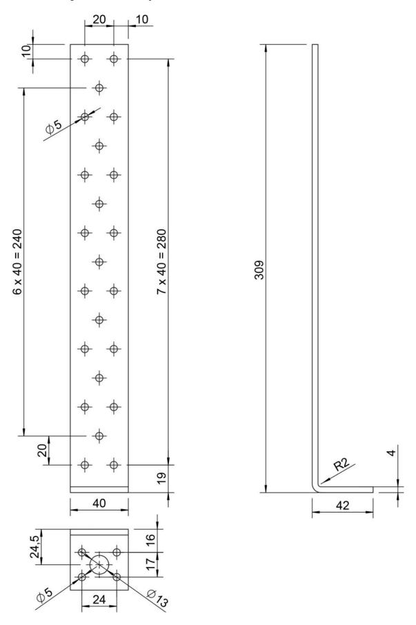
Figure B.54 Dimensions of concrete flat steel anchor 300x40x40x4,0
