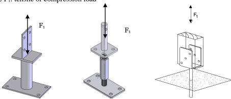
$\bullet$  Force  $F_2$  /  $F_3$ : horizontal parallel to the ground plate of the post base and perpendicular to the bolts or dowels
