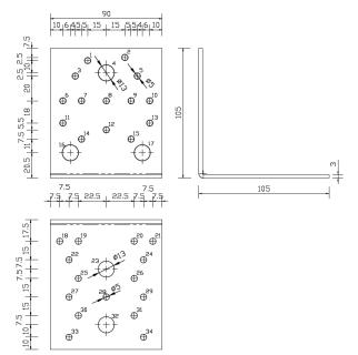
Figure A.5 Dimensions of Angle Bracket 105 with rib
