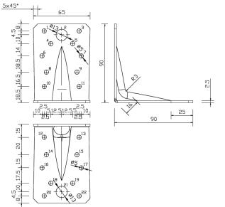
Figure A.3 Dimensions of Angle Bracket 90 with rib
