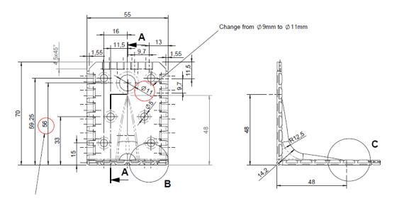
Figure A.7 Dimensions of Angle Bracket 70 with rib, thickness 1,5 mm
