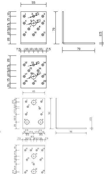
Figure A.4 Dimensions of Angle Bracket 90 without rib
