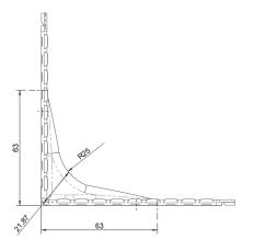
Figure A.9 Dimensions of Angle Bracket 105 with rib, thickness 1,5 mm
